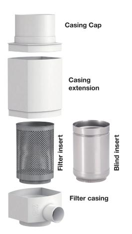
The filter insert: This element is the heart of the RainCollector RS. It is completely made of stainless steel and has a mesh size of only 0,28 mm. Dirt is automatically washed away, therefore it is to a large extend self cleaning.
